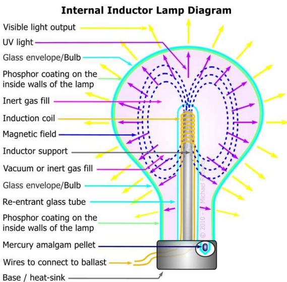
In a variation of this technology, a light bulb shaped glass lamp, which has a test-tube like central re-entrant cavity (glass tube), is coated with phosphors on the inside and filled with inert gas and a pellet of mercury amalgam (see diagram on left). The induction coil is wound around a shaft which is inserted into the central test-tube like cavity and excited by high frequency energy provided by an external electronic ballast, to produce a strong magnetic field.
